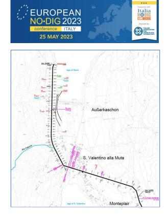
Figure 1. Plan layout of the diversion tunnel
