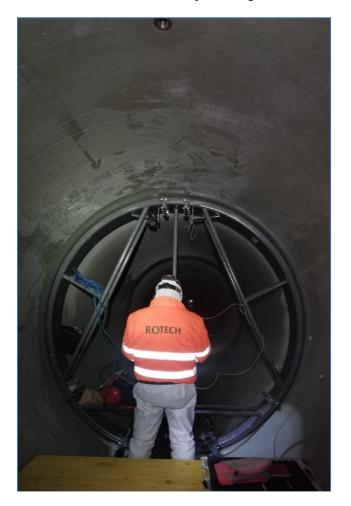
Figure 8. Execution of leak test on single joint
