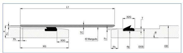
Figure 3. Pipe-sleeve coupling system detail.
