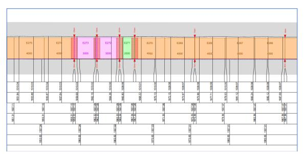
Figure 4. Laying plan for the new GRP pipes marked and numbered
